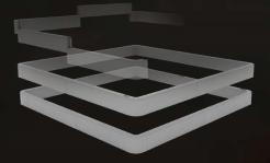
The access pit system features a twinwall sectional design that is made up of GRP corner pieces ('hockey sticks') and sidewall lengths ('straights'). These parts are connected using a jointing peg to form a variety of clear opening sizes. With sidewall lengths being used in conjuction with corner pieces additional access pit sizes specified by the contractor can be made.
